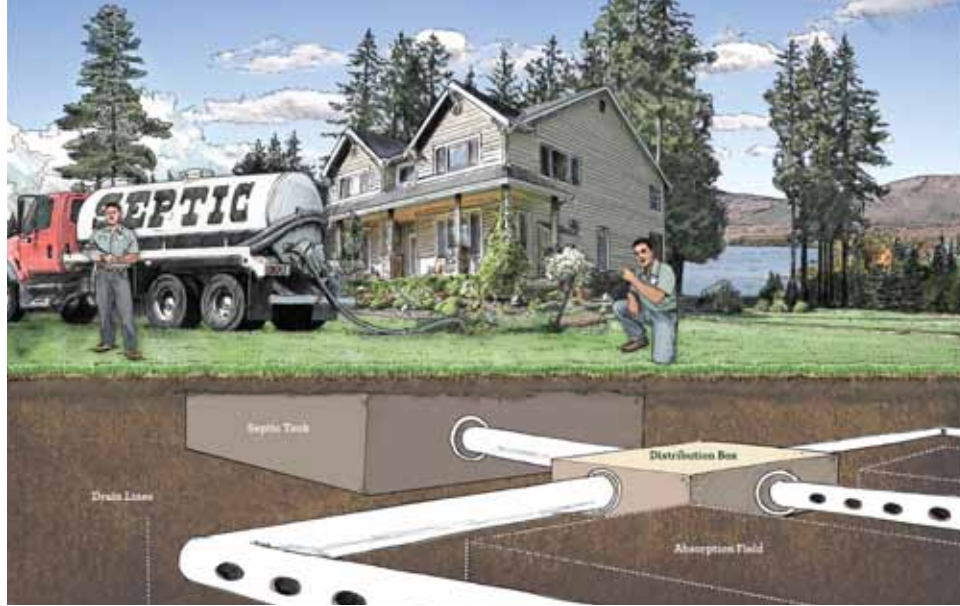
FIGURE 2-2 – Components and Cross Section of Septic System
