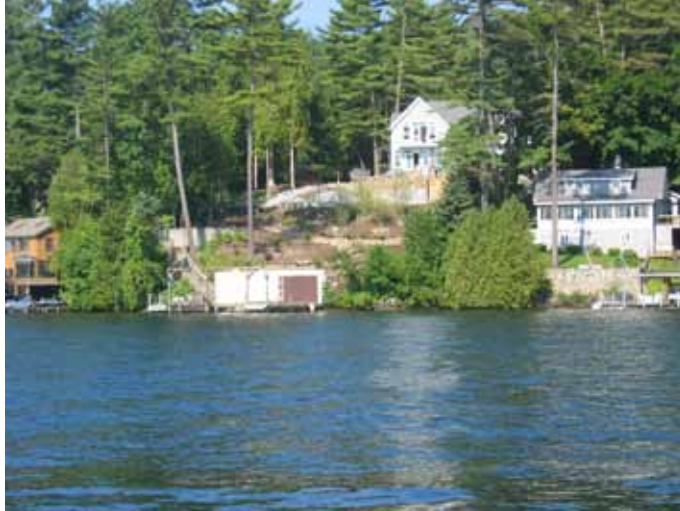
FIGURE 5-1 – Lakefront construction demonstrating difficult site constraints for onsite wastewater treatment systems including setbacks, slopes, and depth to bedrock.
