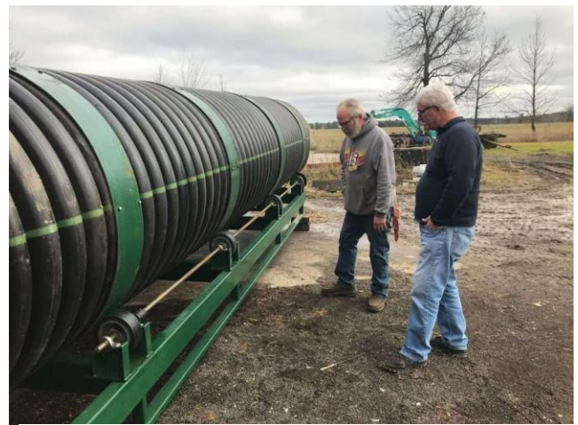
Figure 3-15 In-vessel Drum Composter in the Town of Newcomb
