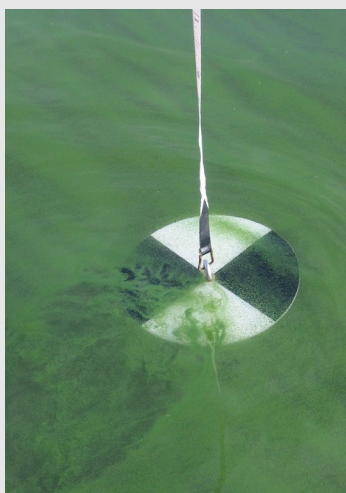
Photo 6: Secchi Disks are used to measure water clarity. Source: USGS.
