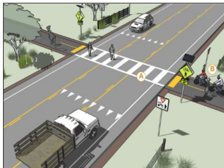
Figure 4-9: Installation Detail for RRFB with Marked Crosswalk (A) and Push Buttons Positioned for Cyclist Convenience (B).
