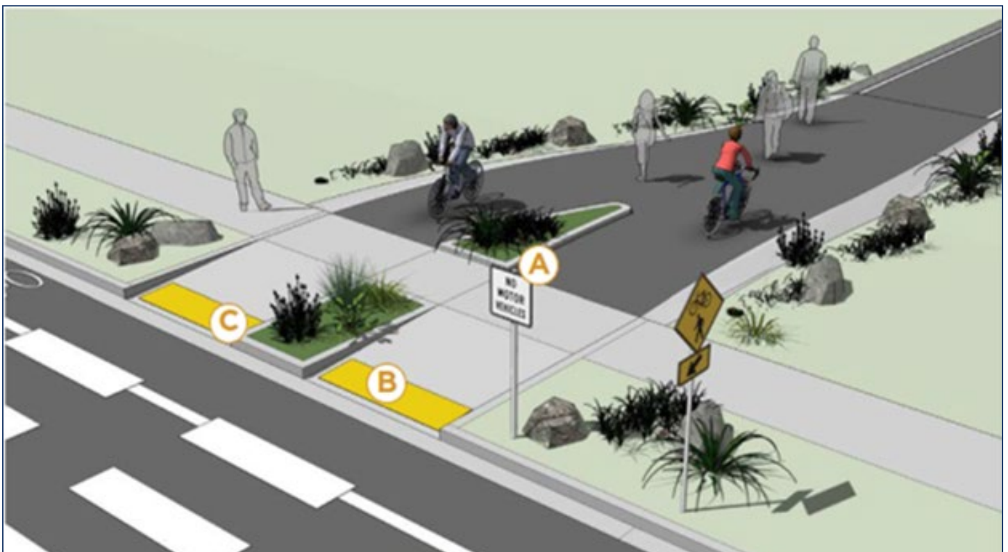
Figure 4-10: Preferred trail entrance/access as outlined in the Empire State Trail Design Guide.
